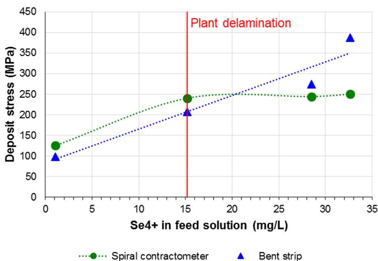
Figure 4. The effect of  $\text{Se}^{4+}$  on nickel deposit stress as determined by the bent strip and spiral contractometer.
