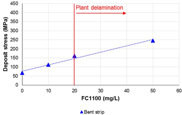
Figure 6. The effect of FC1100 on nickel deposit stress as determined by the bent strip method.
