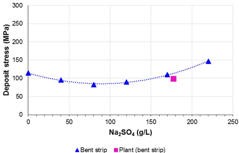
Figure 2. The effect of Na<sub>2</sub>SO<sub>4</sub> on nickel deposit stress as determined by the bent strip.
