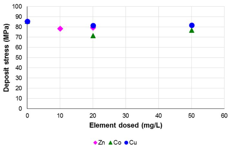
Figure 3. The effect of Zn, Co and Cu on nickel deposit stress as determined by the bent strip.
