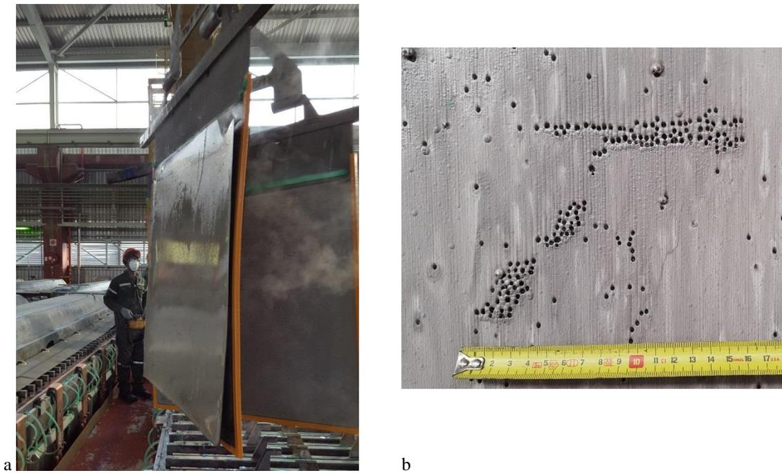
Figure 7. Delamination (a) and “honey-combed” nickel deposit (b) as a result of FC-1100.
