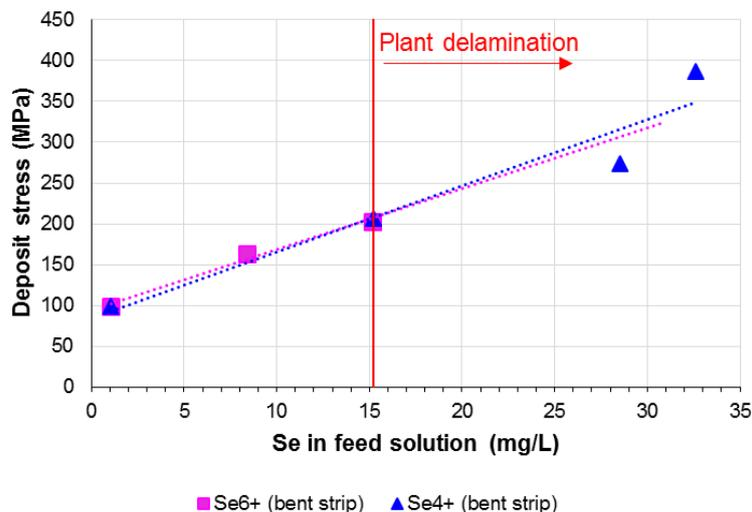
Figure 5. The effect of Se<sup>6+</sup> and Se<sup>4+</sup> on nickel deposit stress as determined by the bent strip.
