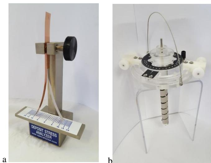
Figure 1. The bent strip (a) and the spiral contractometer (b).
